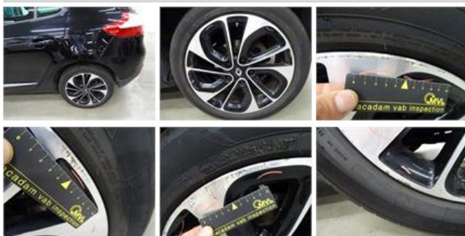
Alloy rim F R polished, Scratch(es), LI - Repair and paint (complete)
