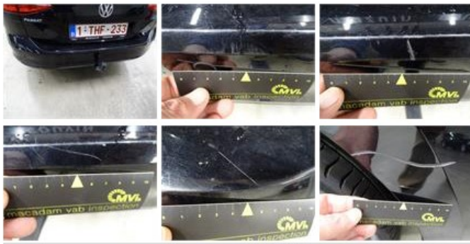
Bumper F, Crack, Le - Replace and paint
