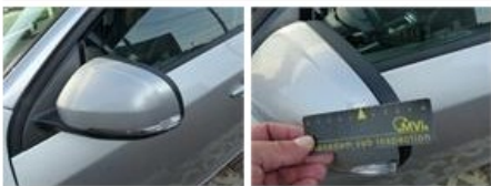
Rearview mirror housing L, Scratch(es), Acceptable
