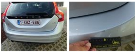
Tailgate, Scratch(es), LI - Repair and paint (complete)
