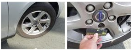
Wheel bolt cover R R, Missing, E - Replace
