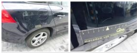
Door panel F L, Scratch(es), Acceptable
