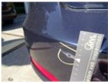
Wing R L, Dent(s), LI - Repair and paint (complete)
