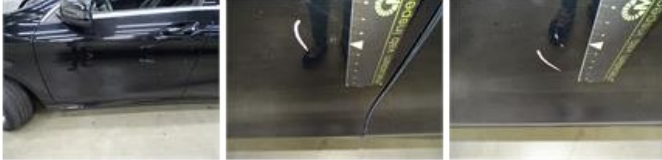
Door F L, Dent(s) and scratch(es), LI - Repair and paint (complete) 318,35
