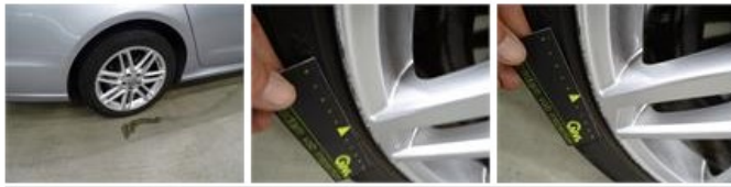
Wing F R, Bad repair, Acceptable
