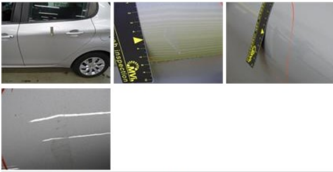
Wheel cover F R, Deformed / Strained, E - Replace
