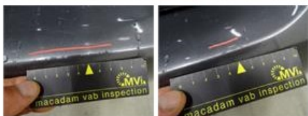
Bonnet, Dent(s), PDR - Paintless dent repair
