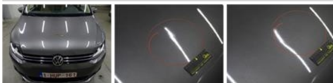
Bonnet, Dent(s), PDR - Paintless dent repair
