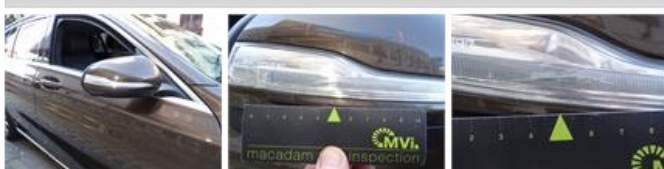
Wing F R, Scratch(es), It - Spot repair
