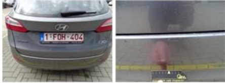
Protection plate M, Deformed / Strained, E - Replace
