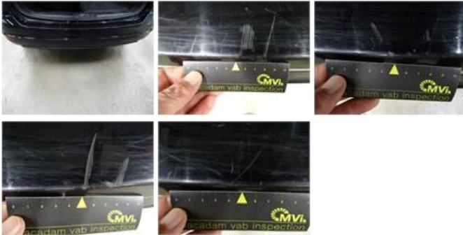
Door F L, Dent(s) and scratch(es), LI - Repair and paint (complete)
