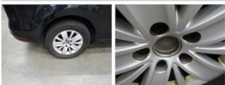
Wheel hub cap R L, Missing, E - Replace 0,00
