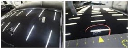
Roof, Chemical polution, LI - Repair and paint (complete) 481,50
