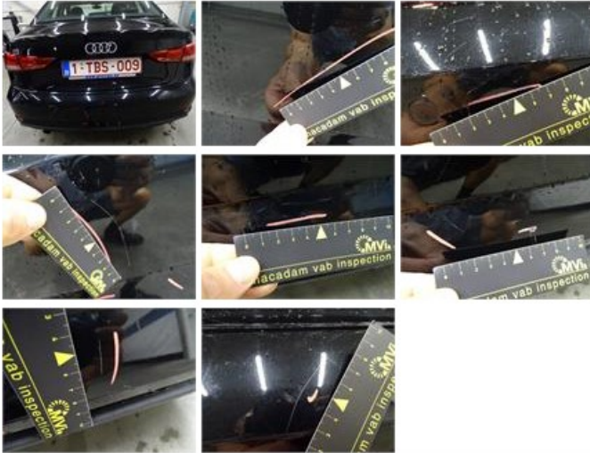
Door F L, Chemical polution, LI - Repair and paint (complete) 318,35
