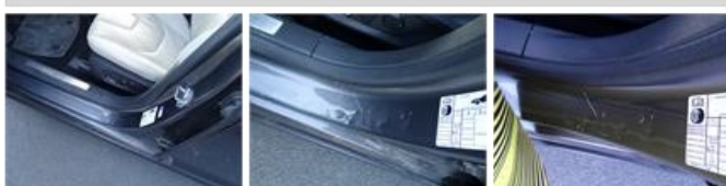
Roof pillar R, Scratch(es), Acceptable
