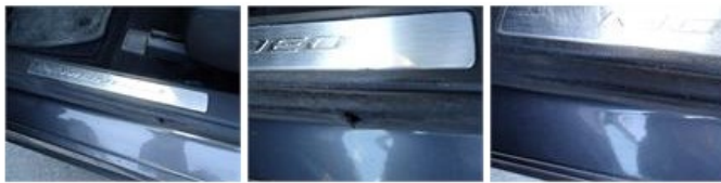
Wing R R, Dent(s) and scratch(es), LI - Repair and paint (partial)
