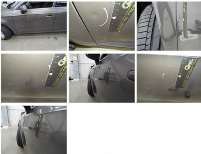
Door R L, Dent(s) and scratch(es), Acceptable
