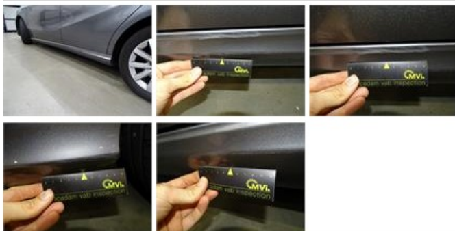
Protection plate M, Deformed / Strained, E - Replace
