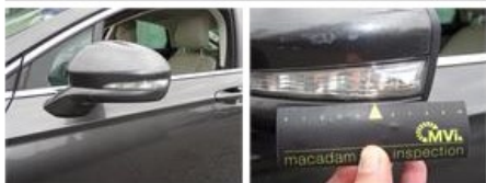
Mirror side blinker L, Broken, E - Replace
