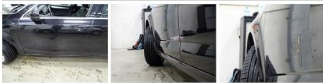
Door F L, Bad repair, Acceptable
