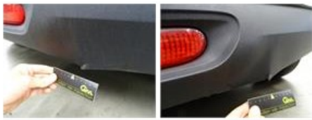
Bumper Trim F, Missing, E - Replace
