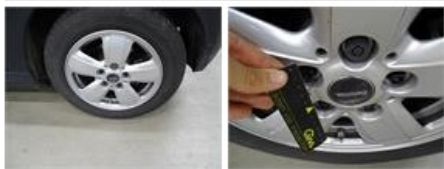
Alloy rim F R, Scratch(es), LI - Repair and paint (complete)
