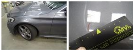
Door F L, Bad repair, Acceptable
