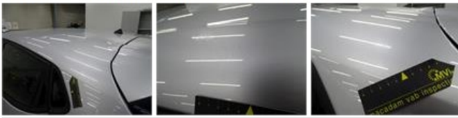
Rocker panel inner F L, Dent(s), LI - Repair and paint (complete)
