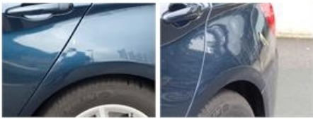
Door F L, Bad repair, LI - Repair and paint (complete)
