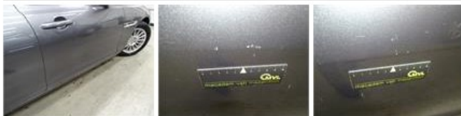
Wing R R, Scratch(es), LI - Repair and paint (complete)
