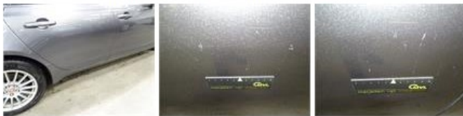
Door F R, Scratch(es), LI - Repair and paint (complete)
