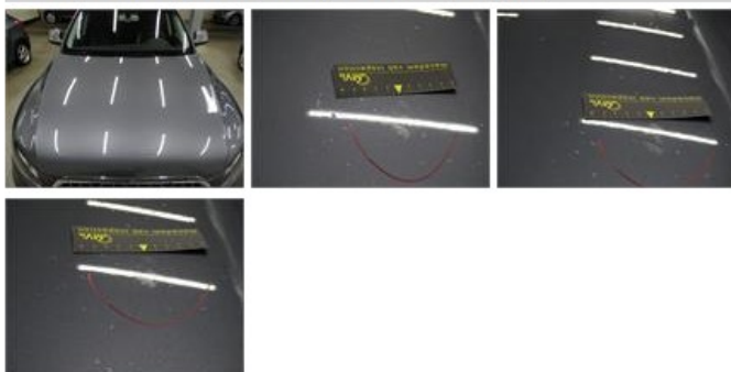
Trunk lid covering R, Scratch(es), Acceptable
