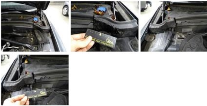
Protection plate M, Deformed / Strained, Acceptable
