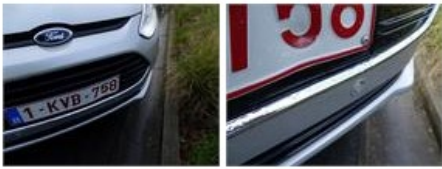
Bumper grille, Broken, E - Replace
