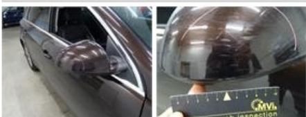
Door F L, Dent(s) and scratch(es), LI - Repair and paint (complete) 318,35
