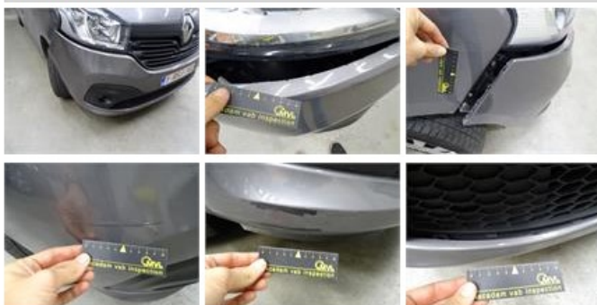
Bumper F, Broken, Le - Replace and paint
