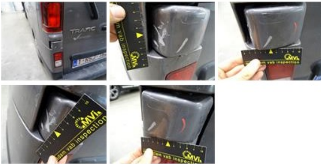
Wing trim R L, Scratch(es), Le - Replace and paint
