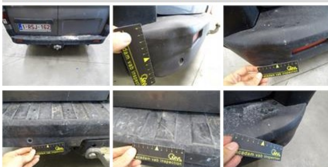
Wing R R, Dent(s) and scratch(es), LI - Repair and paint (complete)
