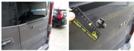
Trunk door R R, Dent(s) and scratch(es), It - Spot repair
