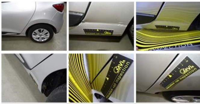
Bonnet, Deformed / Strained, LI - Repair and paint (complete)
