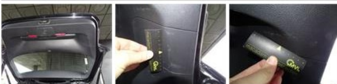
Trunk lid covering R, Scratch(es), E - Replace
