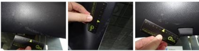
Bumper F, Dent(s) and scratch(es), It - Spot repair
