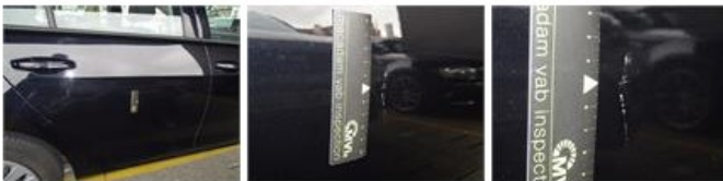
Wing F R, Dent(s) and scratch(es), Acceptable
