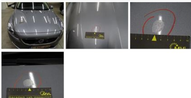
Bodywork, Not original part, Acceptable
