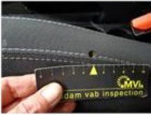
Roof, Dent(s), LI - Repair and paint (complete)
