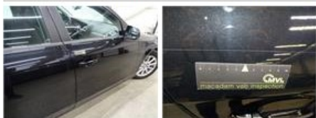
Door F L, Dent(s), LI - Repair and paint (complete)
