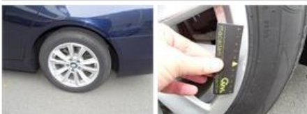
Alloy rim R L, Scratch(es), Acceptable
