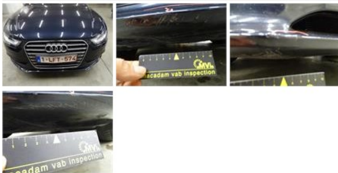
Wing F R, Deformed / Strained, Le - Replace and paint
