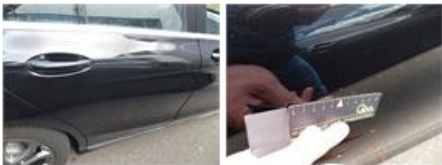
Wing F L, Bad repair, P - Check
