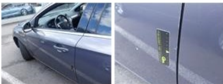
Bumper R, Bad repair, LI - Repair and paint (complete)
