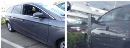
Door F L, Scratch(es), It - Spot repair
