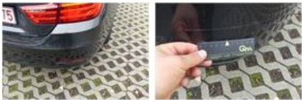
Sill outer R, Scratch(es), It - Spot repair
