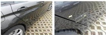
Door F L, Dent(s), LI - Repair and paint (complete)
