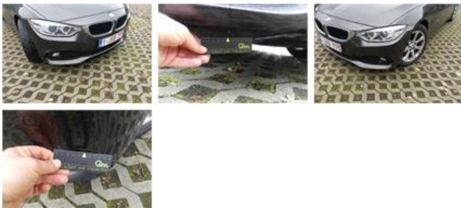
Bumper F, Scratch(es), LI - Repair and paint (complete)
