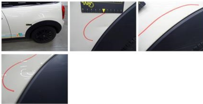
Roof, Dent(s), LI - Repair and paint (complete)
