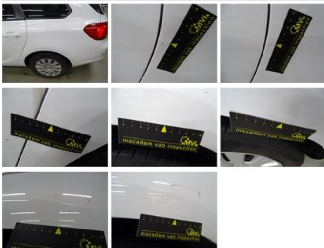
Sill outer R, Dent(s), Acceptable
