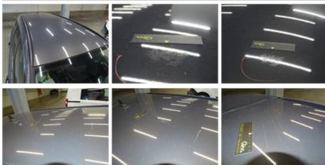
Roof pillar L, Dent(s), Acceptable
