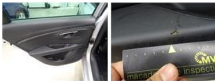
Door panel R L, Tear, Smart repair
