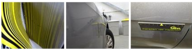
Roof pillar R, Dent(s) and scratch(es), LI - Repair and paint (complete)
