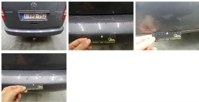
Trunk lid covering R, Scratch(es), Smart repair
