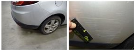
Bumper R, Dent(s), Smart repair
