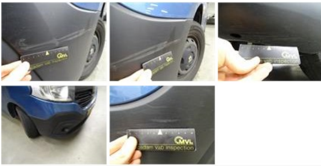
Bumper corner R R, Scratch(es), Smart repair
