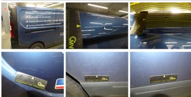
Door moulding Lower R L, Scratch(es), Acceptable
