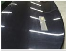
Roof pillar R, Chemical polution, LI - Repair and paint (complete)
