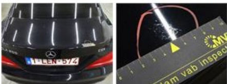
Bonnet, Chemical polution, LI - Repair and paint (complete) 290,08
