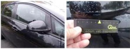
Roof pillar R, Scratch(es), Acceptable
