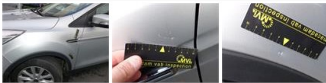
Bumper trim R, Dent(s) and scratch(es), E - Replace
