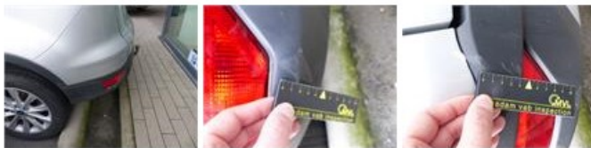
Bumper corner R L, Scratch(es), It - Spot repair
